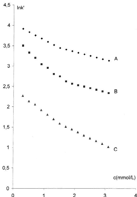
Fig. 3. Plot of  $\ln k'$  against  $c$  for all antihypertensive molecules at a column temperature equal to 25°C: (A) nifedipine, (B) verapamil, (C) diltiazem.
