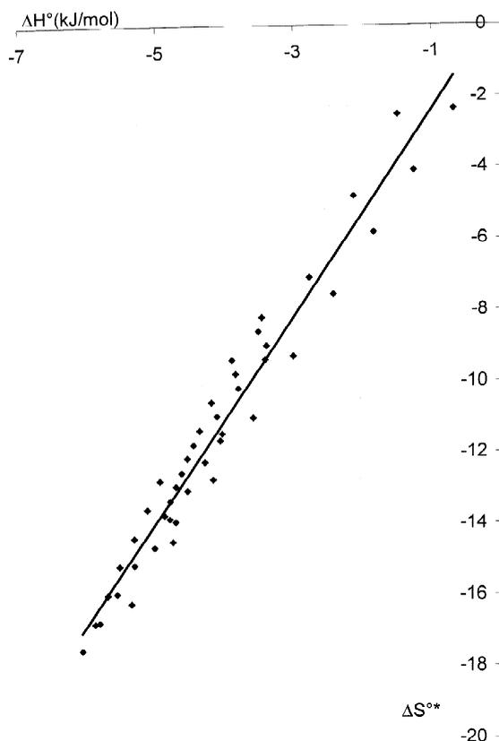
Fig. 6. Enthalpy–entropy compensation represented by the  $\Delta H^0 - \Delta S^{0*}$  plot at the different values of  $Mg^{2+}$  concentration for the three antihypertensive molecules..
